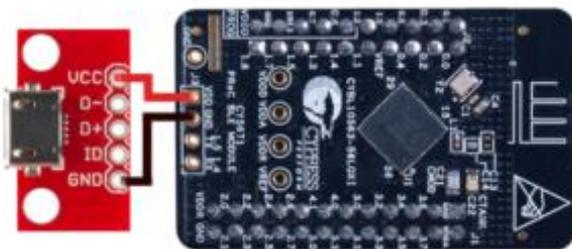
Use two M/M jumper wires to solder the USB board to the PSoC module.
