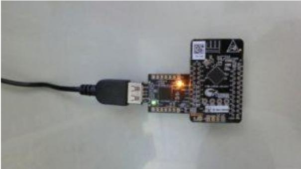
Connect the programming tool to the PSoC and a computer. The location is marked as PROG on the board.
